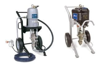
**Minimum Requirements:** 33:1, 100CFM, 120psi constant, 3/4" to 1.25" air delivery line. Air hose feed must be a minimum 3/4" delivery to the unit. 3/8" air hose is not large enough to power the above units efficiently.
